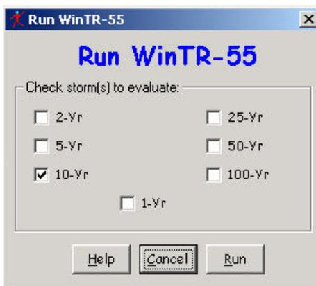
When the “Run” button is selected, after clicking on each desired rain, the program calculates the site runoff and routes it through each reach. An embedded version of TR-20 is actually used to conduct the analyses, being much better than the prior manual TR-55 procedures which required rather crude increments of important site factors. The
